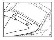
tacts—avoid moving your hands. When your pulse is detected, the heart-shaped indicator in the Calories/Fat Calories/Heart Rate display will flash, and then your heart rate will be shown. For the most accurate heart rate reading, continue to hold the contacts for about 15 seconds.
